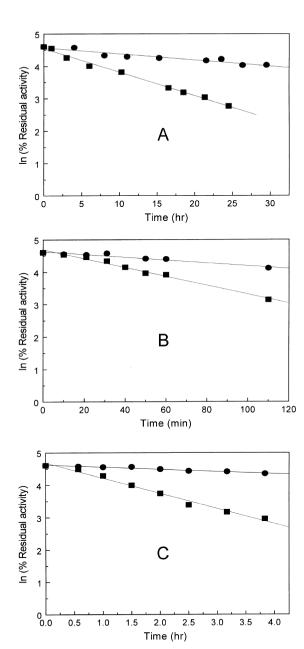
Fig. 4. Stability of the native (■) and the cross-linked (●) enzymes under different experimental conditions. (A) pH 8.0; (B) pH 6.0; (C) in the presence of 20% methanol in 100 mM Tris-HCl buffer (pH 8.0). Data represent an average of duplicate experiments.
