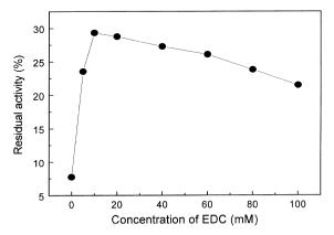
Fig. 2. Effect of EDC concentration on the activity of D-hydantoinase. After the cross-linking reaction, the enzyme solution was incubated at 70°C for 1 h, and then the residual activity was determined. Data represent an average of duplicate experiments.
